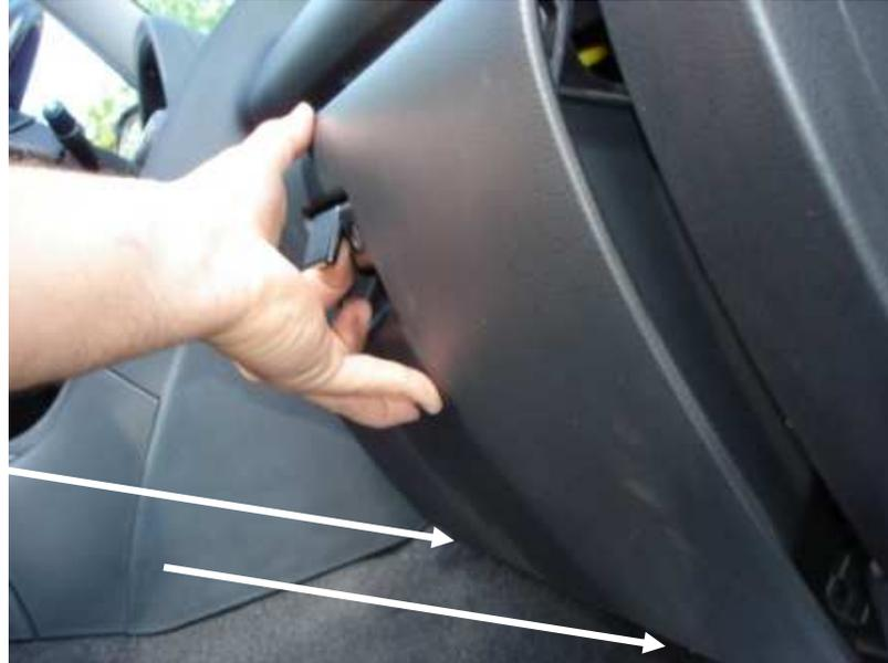
**Step 2:** Use the needle nose pliers and gently squeeze the plastic end on the pin which is split, and slide the pin through the hinge. This might be easier with the help of a screwdriver. Do not remove it, but just clear it of the hinge.
