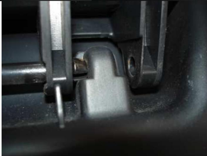
**Step 3:** Now open the glove box, and tilt it towards you (as you are sitting on the passenger side door sill) and remove it. It will take some maneuvering to get it out, but rotate it and you will clear the rubber stops allowing the glove box to come out.
